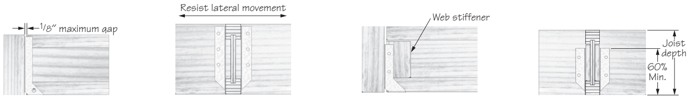
(Top flange support requirements can be verified in EWP Top Mount Hangers charts under the Web Stiffener Req. column of USP's Full Line Catalog .)
